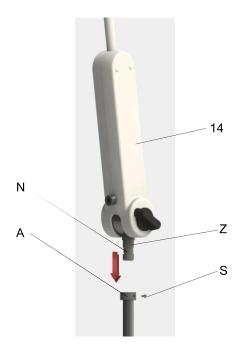
Tighten screw **S** in the mounting device (stand, wall, table, rail, round and rectangular tube, screw-on plate) after the lamp has been attached. This prevents the lamp from being unintentionally removed.
